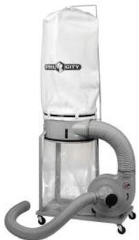
Dust and chip collection can be done with: a small shop vac, which moves a high volume of air quickly over a small area; dust collector or cyclones which move large volumes of air at a slower velocity, but greater area. The air born dust can be pulled from the air with separate air filters, or filtered out by your dust mask, and then you will need a broom to get the chips. Don't work without some sort of dust collection or filtering if you are generating dust.
