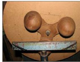
Robbie has taken and cut away much of the support material between the bowls, and then remounts the piece and does the final clean up turning.
