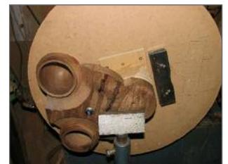
Once each bowl is finished, the blank will need to be flip over to turn the top surface. To help hold the blank in place, Robbie places the bowl being turned in a wooden chuck fastened to the backer board to support the piece. Once all the rough turning is done, the piece can be removed and trimmed up to a final shape.
