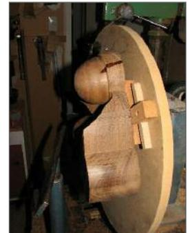
The blank is firmly bolted to the carrier board which is fastened to a large face plate on your lathe. The blank is initially centered on the backer board to allow turning out most of the center material. It is then positioned offcenter so that each bowl will be centered on the backer board so that they can each be turned.
