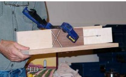
With the veneer inserts ready, it is time to start to cut up your main stock. He uses a chop saw for all his cuts and has made a simple jig to hold the blanks properly during cutting. This allows the small cut off to safely fall away without becoming jammed between the blade and stop block. For him, a piece of paper and a pencil are used to draw a scale sized blank, and then draw on the
