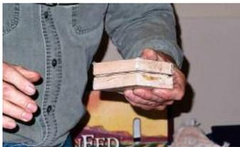
To help in the assembly of the pieces, he sizes and glues up the veneers and presses them between a set of culls wrapped in wax paper until they are dry. Plenty of clamps at hand are a good thing to help spread the load evenly over the veneer so that they bond well and are the same thickness across the entire piece. You will need 4 separate
