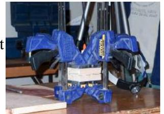
pieces of finished veneer insert ready to go to make the knots, and they all need to be the same thickness.
