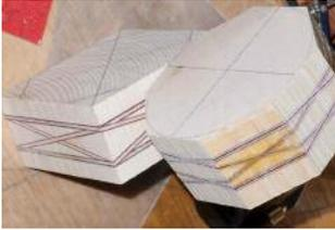
To make a successful knot pattern, the thickness of the material removed by the saw blade during the cut needs to be replaced, and Carl glues up veneers to fill that gap. All the examples he brought along had contrasting colors in the veneers so that they really stood out in the piece.
