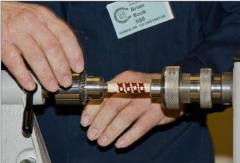
You need to have the ends of the pen blank square to the tube, and to help keep the tubes straight, he used the insert portion of a pen mill in a Jacobs chuck. The pen mill shaft just fits inside the tube and allows the tube to freely rotate on the end of the mill steel. For the sanding, he has devised a small sanding disk for his head stock mounted collet chuck to clean up the ends of the blanks.
