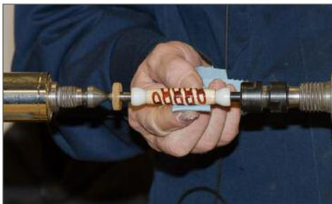
between the delrin bushings, it is centered along the lathe axis, and the CA glue does not stick to the synthetic bushings.
