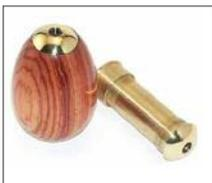
Carl turned a simple egg kit kaleidoscope to start off to show the simplest form. It is a simple body with prepackaged parts that slide into the turned body. The kits are available from places like Lee Valley and Craft Supplies.
