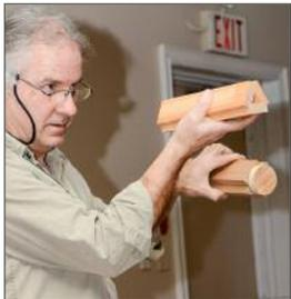
Once the end caps are done, it is on to the body. For that, Carl glues up a series of staves to allow for a fancier look. You can use different colored woods or a series of glued up pieces to make each side. To help hold it on the lathe while turning, he glues on a simple end cap that will be parted off later. The triangular space inside the body will be used to support and hold the mirrors.
