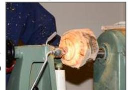
Eugen drills a pilot hole that will be used for hollowing out the inside of the vessel. For this he has found that the Maxi-Cut Forstner bits with their additional scoring spurs make quick work of the material on end or side grain. Once there is a central hole to work from, Eugen has a varied arsenal of hollowing tools to try and help him get to the finished pieces.
