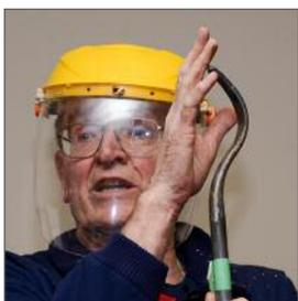
Most of his hand held hollowing tools for vessels are large to try and reduce the vibration while cutting. He generally starts with a goose neck hollowing tool to clear out the material inside the vessel. This works well if the tip is inline with the main shaft. If it is not inline, then there will be a rotational torque on the tool end, making it hard to hold.
