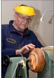
Once you flip the piece around and mount it in the chuck jaws on the tenon, there will be a little bit of wobble, so if you are thinking about doing any sort of decoration on the outside, now would be the time to do that before mounting the tenon in the chuck, while the piece is running true.
