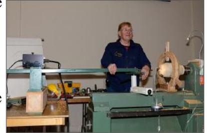
He has added a fiber optic light source that can be attached near the cutter head to allow him to see into the vessel as he cuts and depending on the depth of the vessel, a bowl steady can be added to the mix for extra support of the spinning vessel.
