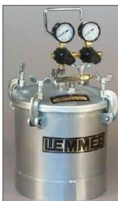
With the resin and mold placed under pressure, the air bubbles and cavities get compressed and the resin gets pushed into those cavities. Your mold though needs to have some additional things that you may not normally think about. You need to provide routes for the resin to flow through to allow it to get to your entire piece.
