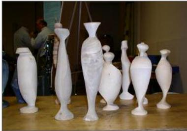
He demonstrated how with 2 centers on each end that are a bit off set from each other, how the tool cuts a curved surface on the work piece even as you move it straight across the tool rest. He showed how the surface changes as the pair of centers move relative to each other. When you start to understand the relationship between the offset centers, you can then plan the final twisting shape.
