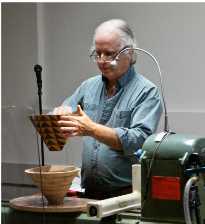
Carl then got onto the demonstration for the night, dizzy bowls. These are primarily bowls from a board that are constructed from a laminated board of differing wood species. As Carl mentioned, his first bowl was just laminated from whatever he had in hand and with no thought to symmetry of the laminations, however, it still produced a striking pattern of a bowl. The trick is to glue the layers up with a slight twist to each layer compared to the previous one.
