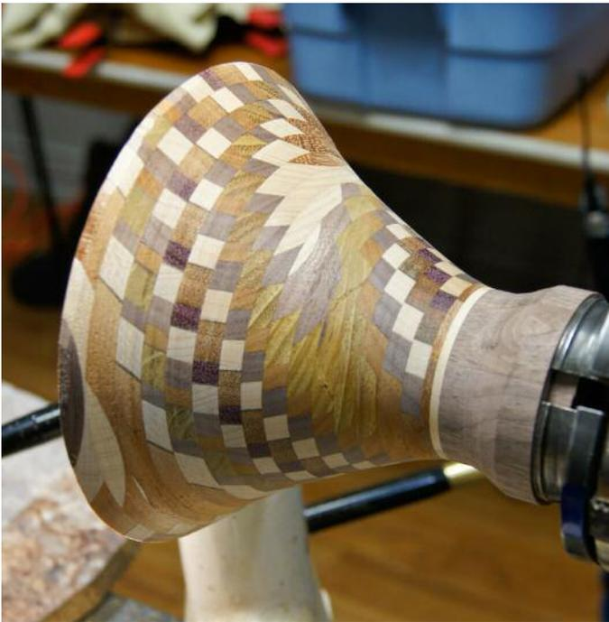
As the layers are gradually built up, he would then smooth out the exterior and then turn the interior – doing the interior after a few layers so that he did not have to extend too far over the tool rest. As the bowl got bigger, he would use a steady rest to finish the inside and an auxiliary centre for finishing the outside.
