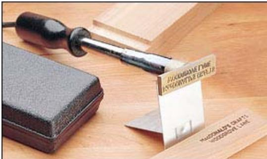
When the branding iron reaches the proper temperature (about 800° F) – usually determined by testing a piece of scrap material – you simply press it against the work for about 1 to 2 seconds and your piece is permanently marked. It's that simple.
