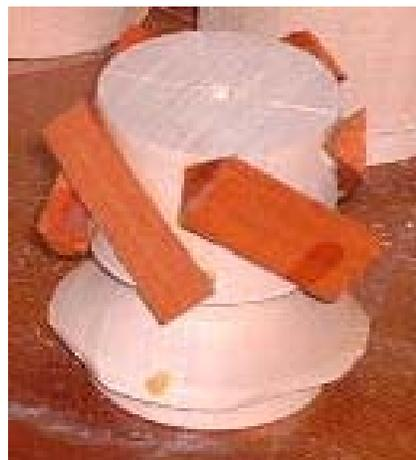
The glued inlay piece was re-mounted in the lathe and brought down to a cylinder. Made a flat spot for the finial to mate with and defined the center before drilling to ensure an inline hole. He drilled out the center and did not consider it worth hollowing out the center since the ornament was quite light when finished.
