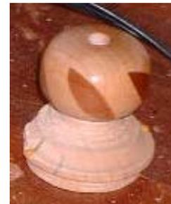
After finishing the top of the ornament Jack polished with Mylands friction polish and parted off the piece.
