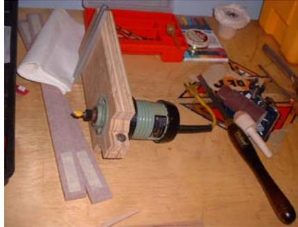
He mounted the jig on the bed of the lathe and the router was setup with V-groove 90 degree bit. Grooves were cut into the orna-
