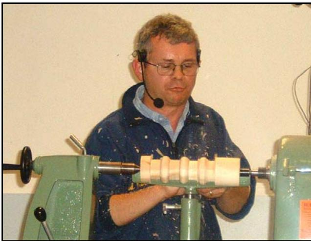
The **Roughing Gouge** is a very versatile tool that can be used for 95% of spindle work. The roughing gouge is available in a wide range of sizes and mostly used to quickly bring square stock to round.
