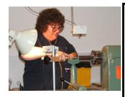
(Ensure the lathe's tool rest is smooth before turning on the lathe. Every nick will be transferred to the work piece!).
