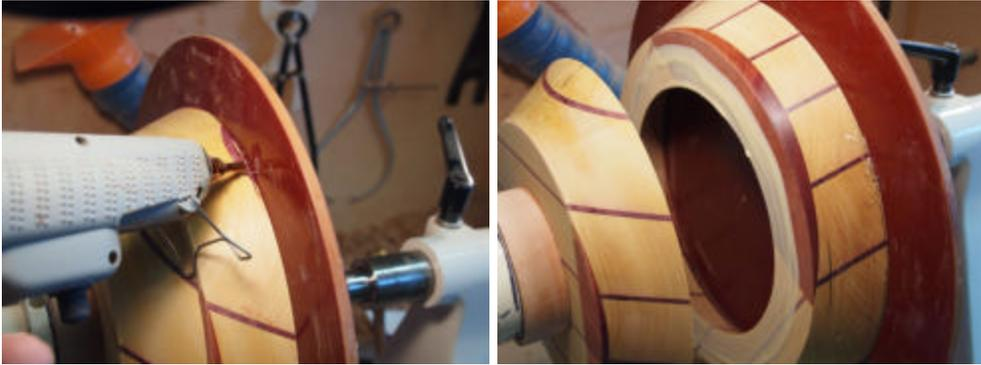
Do each layer the same way until done. Depending on the glue used allow each layer to dry about 1/2 hour and then all layers clamped over night before machining.
