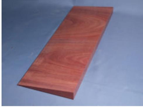
Any tear out on the trailing edge is cut off when roughing out the circle on the band saw. The wedge should be oversized and at least 1/8 thick at the thin edge. An edge too thin can wrinkle with the moisture in the glue and leave a ragged edge when resurfaced. Note the grain orientation of the wedge. It should be the same direction as the blank to avoid cross grain glue joints.
