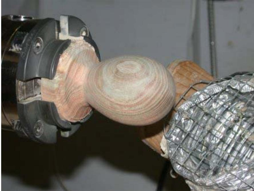
Stage 1 Turning completed prior to finishing
