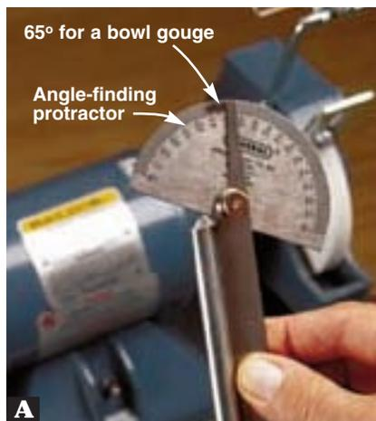
rest, position its leading edge about 1/8" from the wheel. Make all jig adjustments with the grinder stopped.
