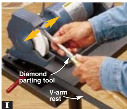
Flip the tool over frequently, lightly grinding both the point's edges until the ground faces intersect at the wide center of the tool. Due to the curve of the grinding wheel, you'll get a point with a slight hollow grind, as shown in the drawing. ♣
