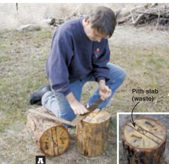
A To remove the pith and a large-diameter unstable zone around it, draw lines with a permanent marker to guide your cuts. The slab marked here is about 1¼" wide.
